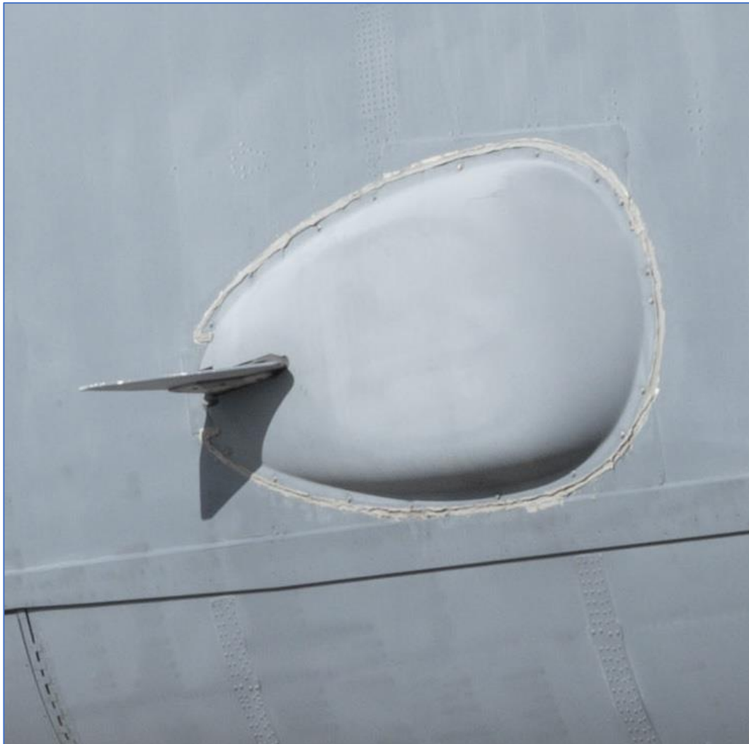
Figure 3. Close-up of starboard side 'New START fin' in place on B-52H 60-0059
