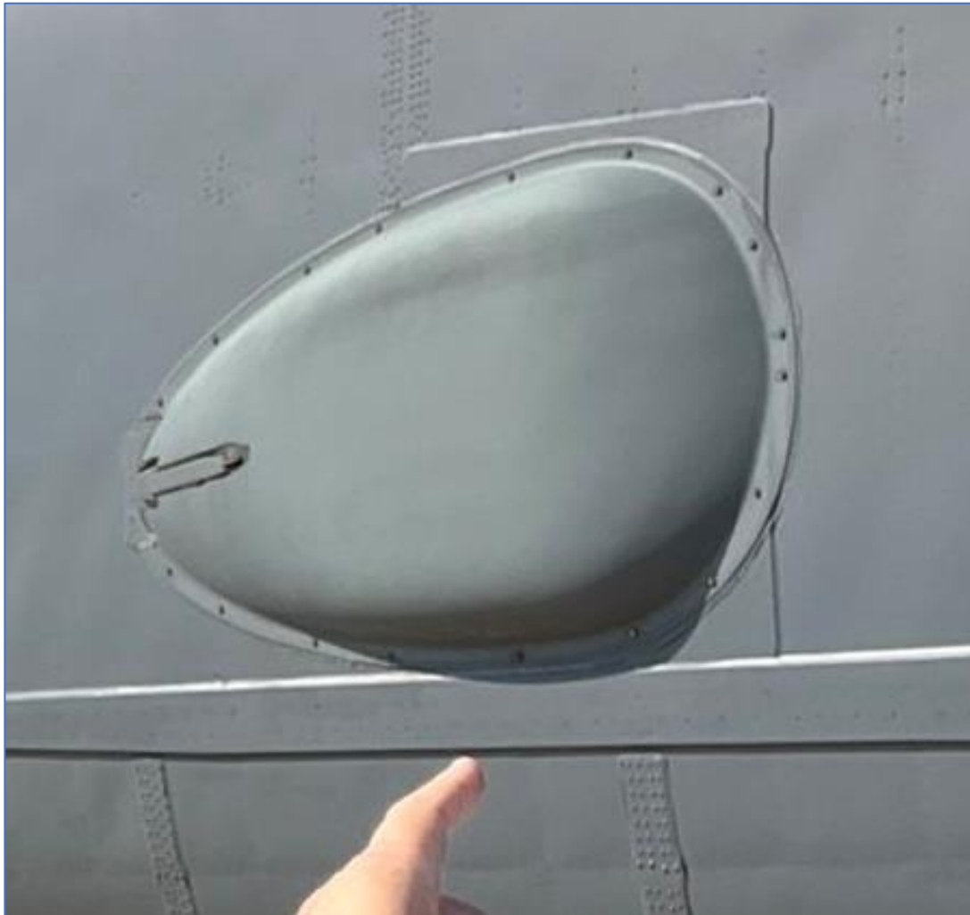
Figure 4. Absence of ‘New START fin’ on B-52H 61-0021 indicating conversion to conventional-only armament
