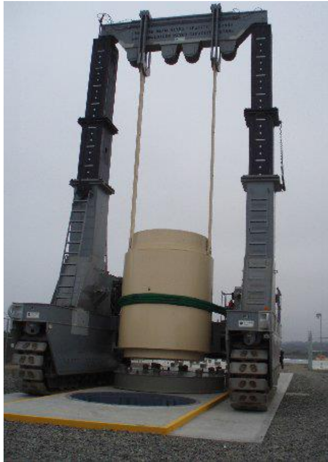
Figure 2-9: Vertical Cask Transporter in Use at Humboldt Bay (California, USA) Interim Storage Site 22
