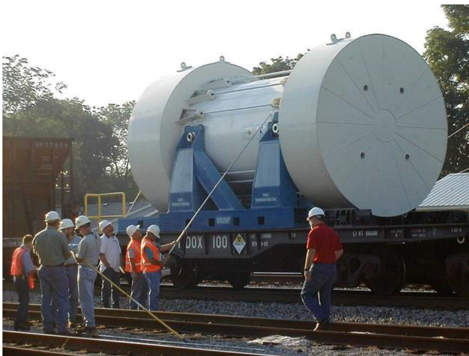
Figure 2-7: Example of Rail Car Carrying Spent Fuel Cask 20
