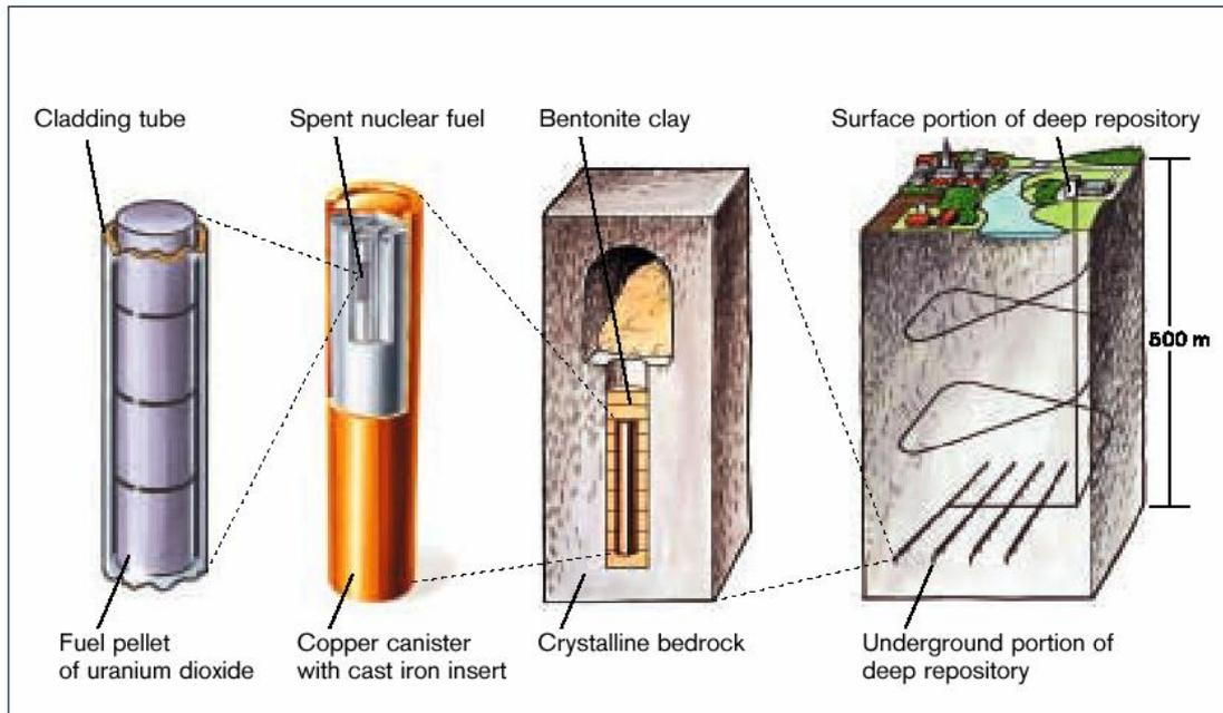
Multiple barriers prevent the radionuclides from reaching the ground surface.
