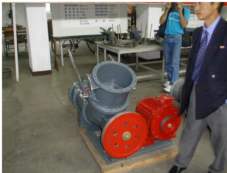
Figure 4-1: DPRK-made Mini-Hydroelectric Turbine-Generator 41
