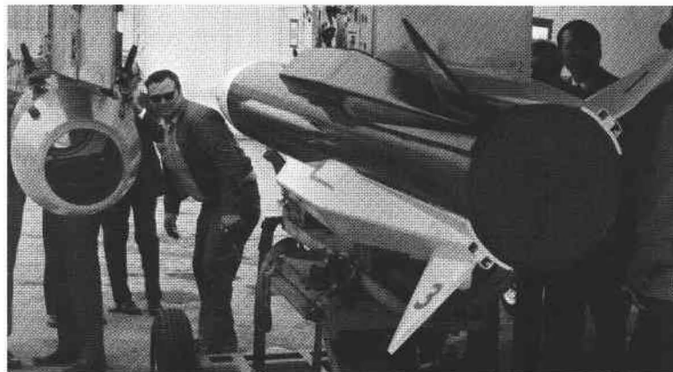
STV-1 Air-Launched Low-Volume Ramjet on A-7A aircraft (1974).
