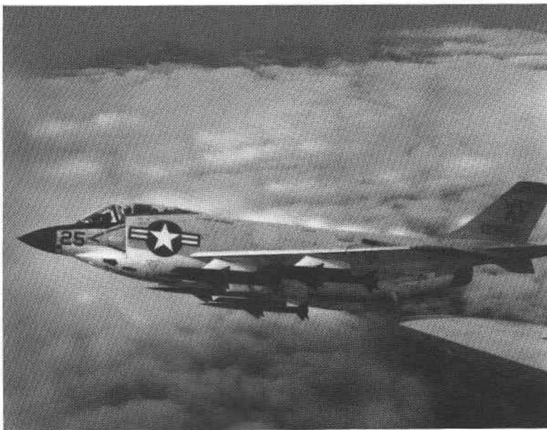
F3H-2N aircraft with SPARROW I missiles on wing pylons (1956).
