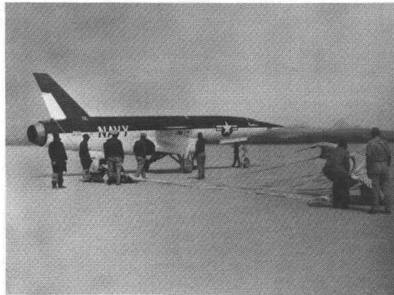
Collapsing a brake parachute after REGULUS II recovery (1956).
