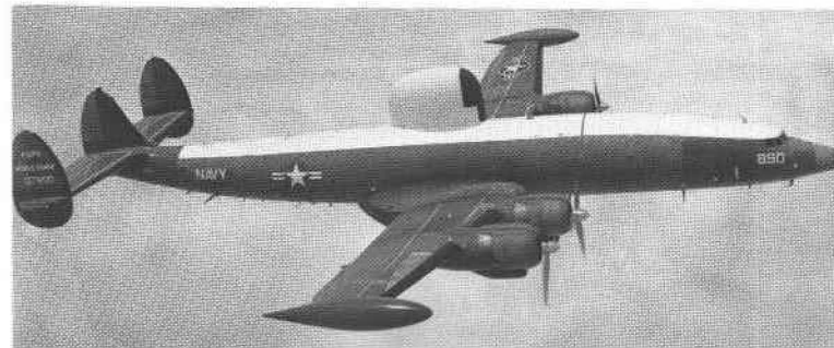
WV-2 (EC-121) Constellation, a range instrumentation aircraft.
