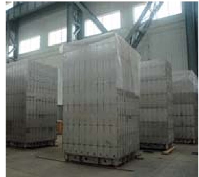
Borated stainless steel frame for SF high-density storage.
