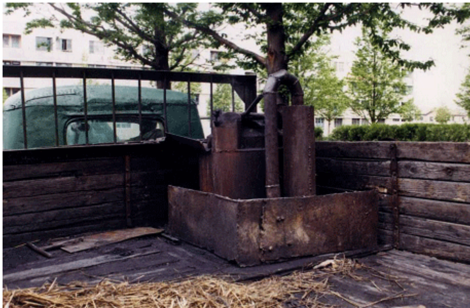
DPRK truck powered by a coal (and/or biomass) gasifier. Source: Nautilus Institute
