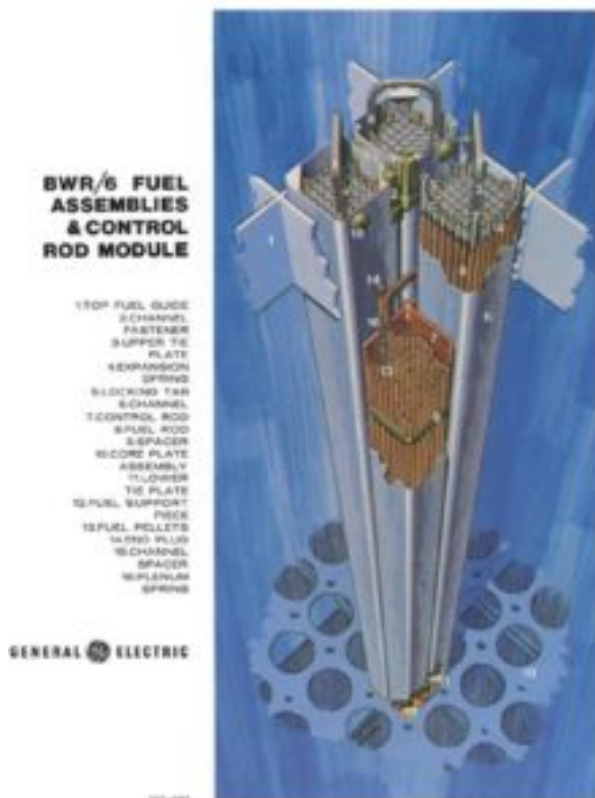
Figure 7: BWR fuel assemblies, showing the metal sheath surrounding the assemblies. From NRC, undated.
