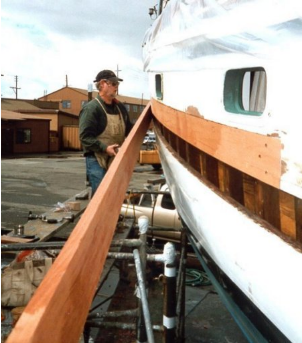
Master boat builder Jim Linderman checks the fit of a new plank he constructed from mahogany.
