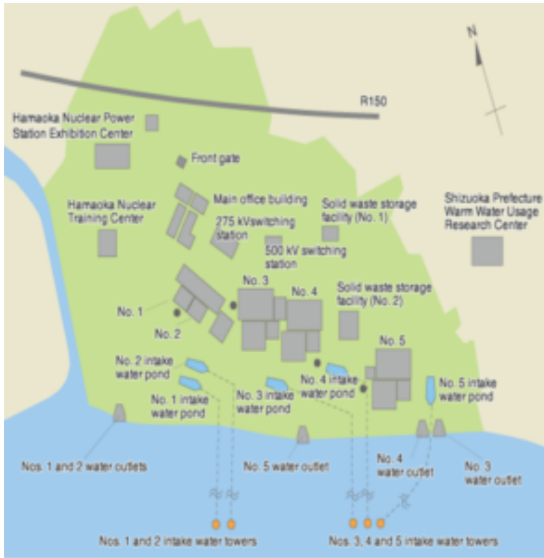
Figure 2-1: Diagram of Hamaoka Nuclear Power Plant[6]
