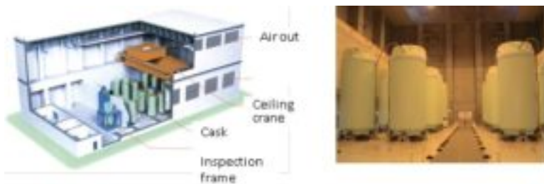
Figure 4: Design concept of cask storage facility to be installed by Japan Atomic Power Company, and the layout of the storage-only casks in the facility (Provided by Japan Atomic Power Company)
