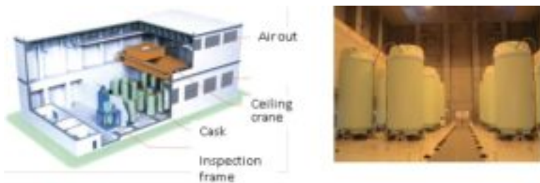
Figure 4: Design concept of cask storage facility to be installed by Japan Atomic Power Company, and the layout of the storage-only casks (Provided by Japan Atomic Power Company)
