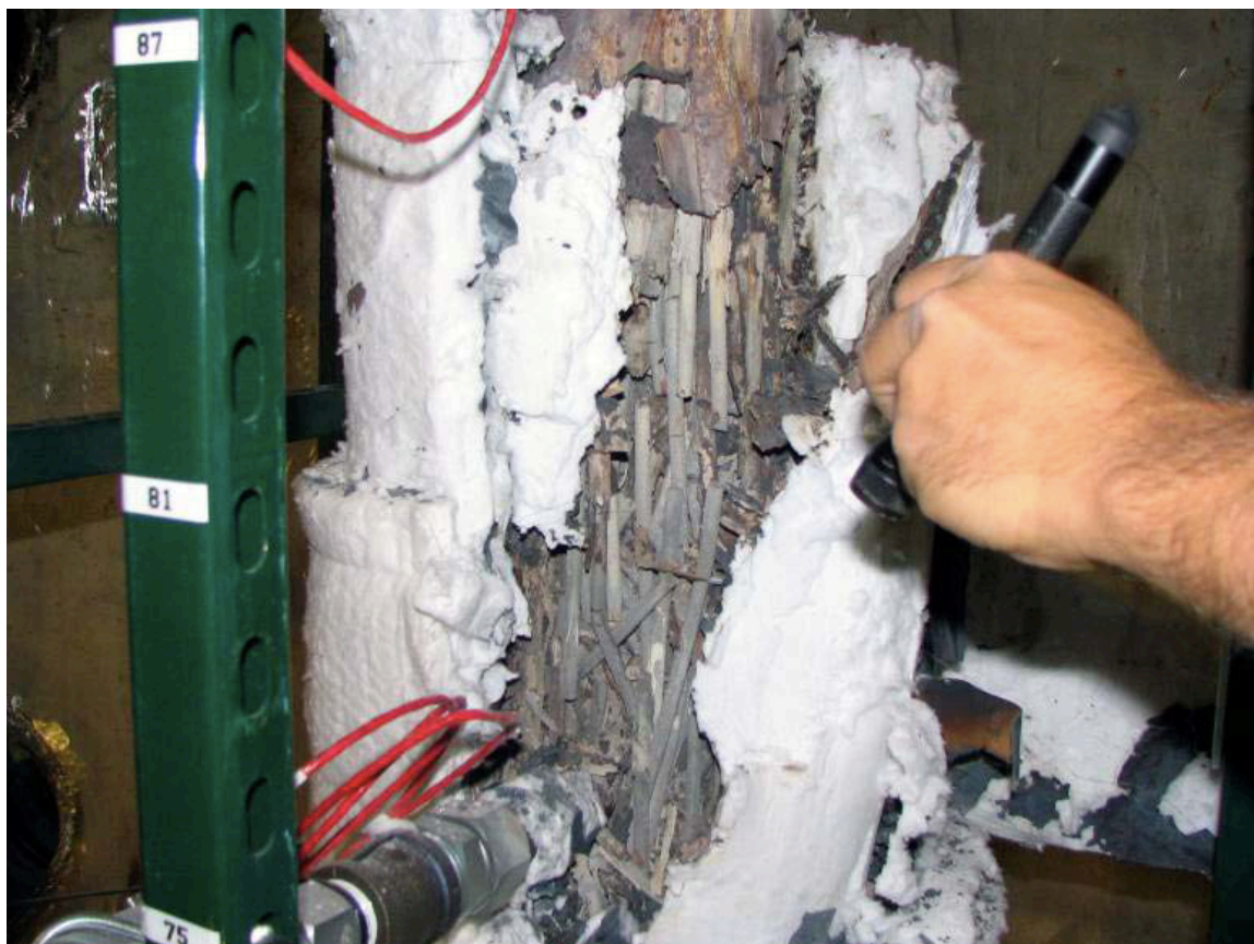
Figure II.3-3 Outcome of Test Burn of a BWR Fuel Assembly
