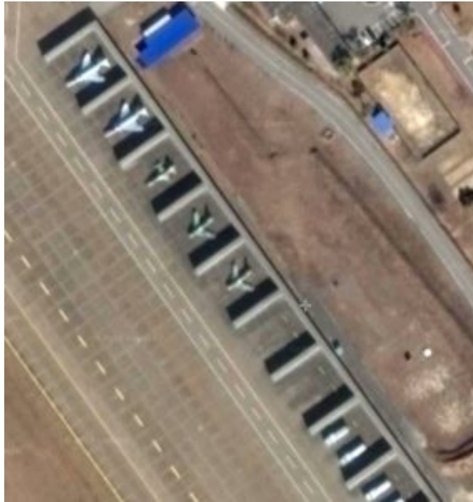
Figure 4: Open revetment storage at runway.
