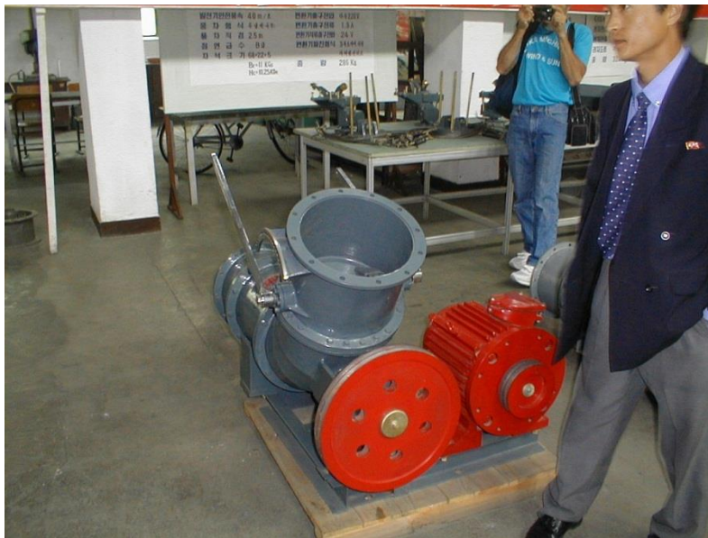
Figure 4-1: DPRK-made Mini-Hydroelectric Turbine-Generator 41
