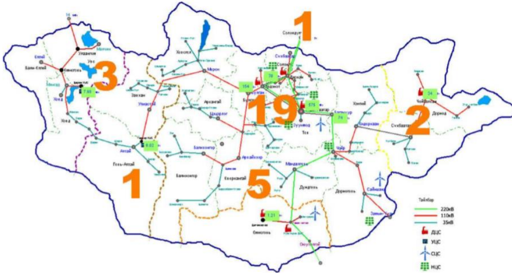
Figure 3: Data collection points of the Mongolian SCADA system
