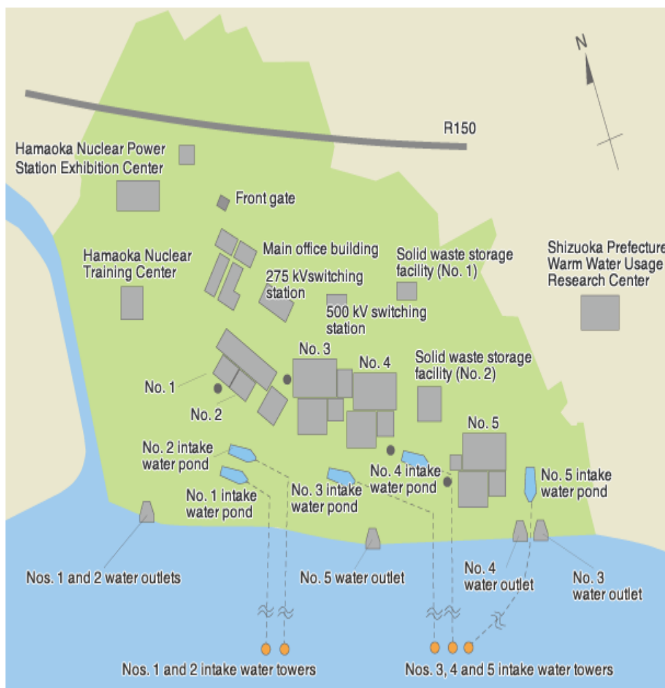
Figure 2-23: Diagram of Hamaoka Nuclear Power Plant 39
