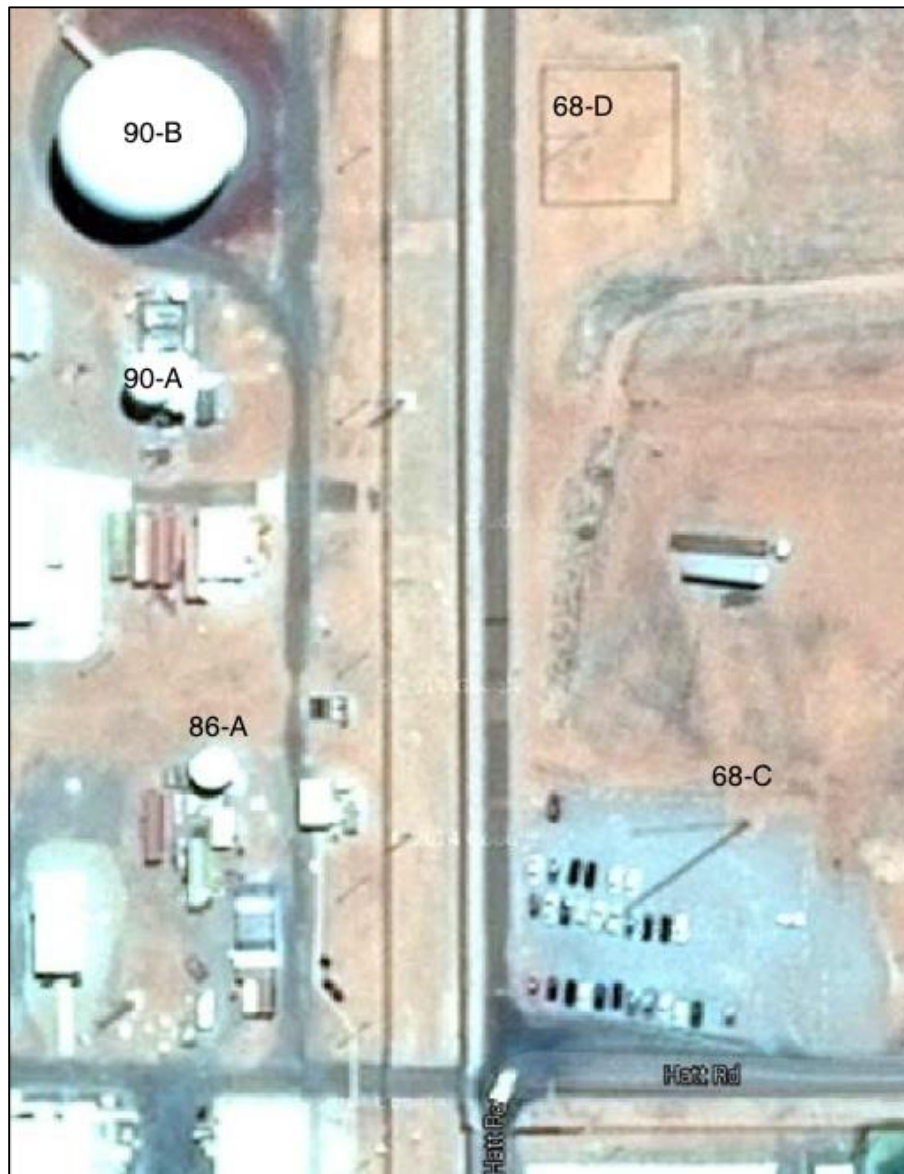
Figure 11. HF transmitter (68-C) and receiver (68-D) antennas at Pine Gap, Google Earth imagery, 6 November 2015
