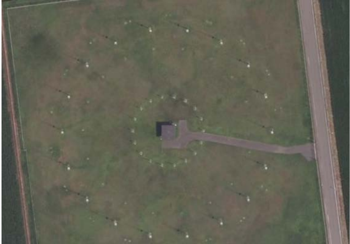
Plate 62 36-element CDAA, Kobunato, Bing imagery, 2009. (Replaced by a 7-element CDAA in 2010)
