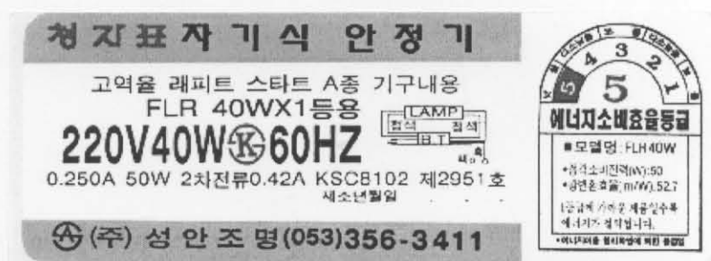
Figure 5-12. Energy label for a fluorescent ballast in the Republic of Korea
