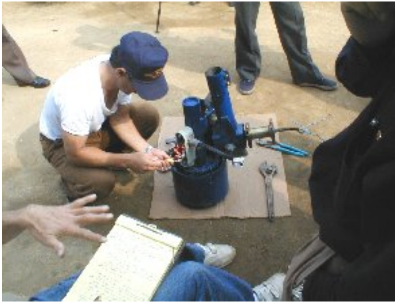
Reassembling 3-Kilowatt Turbine
