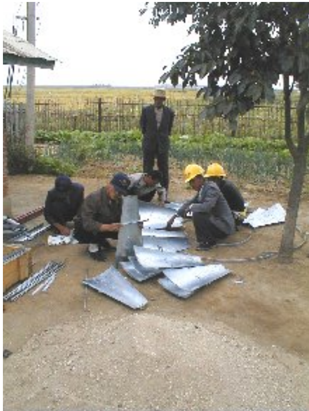
Assembling the Blades for the Windmill
