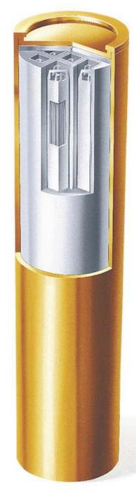
Spent fuel in cast iron insert inside copper overpack (c.5 metres long)
