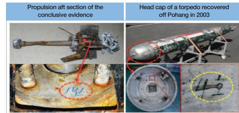
〈Figure III-8-7〉 The Korean inscriptions on torpedo propulsion motor and North Korean light torpedo
