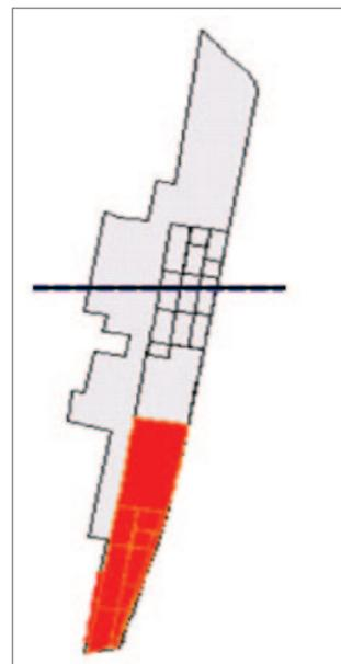
〈Figure Appendix VI-4-7〉 Buoyancy level with four compartments flooded(Case 6)
