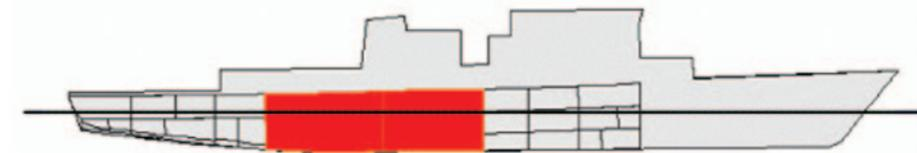
〈Figure Appendix VI-4-1〉 Buoyancy level with 2 compartments flooded(Case 1)
