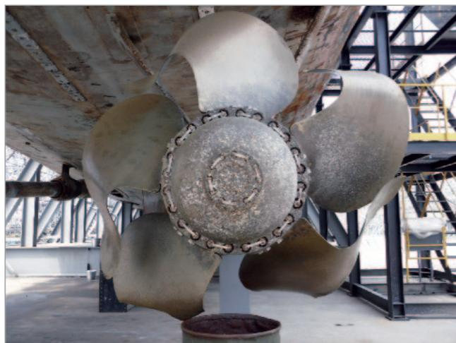
〈Figure II-1-7〉 The deformation of starboard propellers
