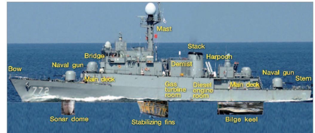
〈Figure I-4-1〉 Overall shape and structures of ROKS Cheonan
