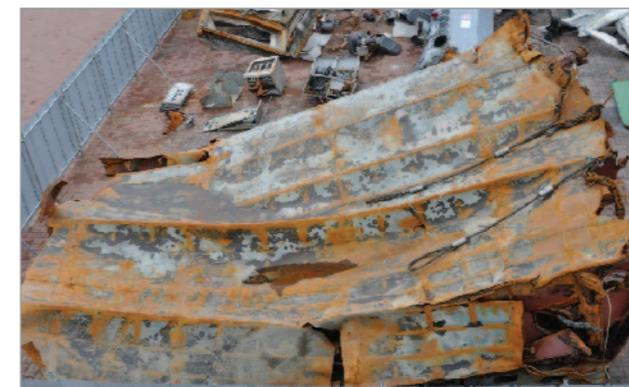
〈Figure II-1-5〉 Shell plates of ROKS Cheonan gas turbine room
