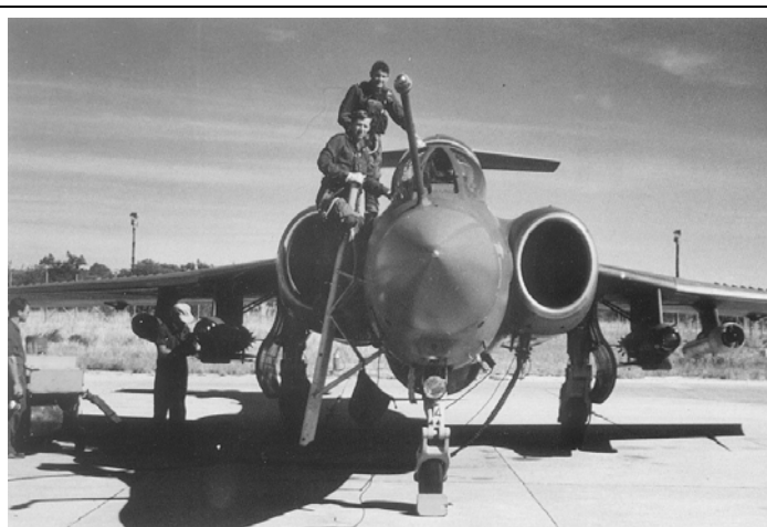
Figure 2: SAAF Buccaneer S Mk 50 aircraft armed with two H2 long-range precision-guided weapons.
