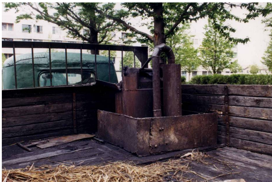
Figure 2-20: Photo of DPRK Truck Powered by a Coal (and/or biomass) Gasifier 127
