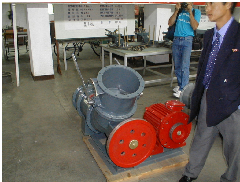
Figure 6-1: DPRK-made Mini-Hydroelectric Turbine-Generator 197
