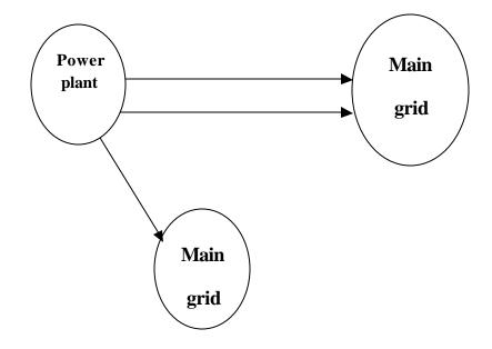
The Tieling power plant has two 300MW generators connected with the main grid through one 500kV line. The Shuizhong power plant has two 800MW generators connected with the main grid through one 500kV line to the North China grid and two 500kV lines to the Northeast grid.
