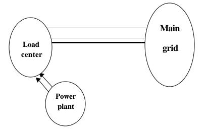
Load center is connected with the main grid through one 500kV line and three 220kV lines. When the 500kV line faults or needs repairs, the active power at one 220kV line will be beyond its limit.
