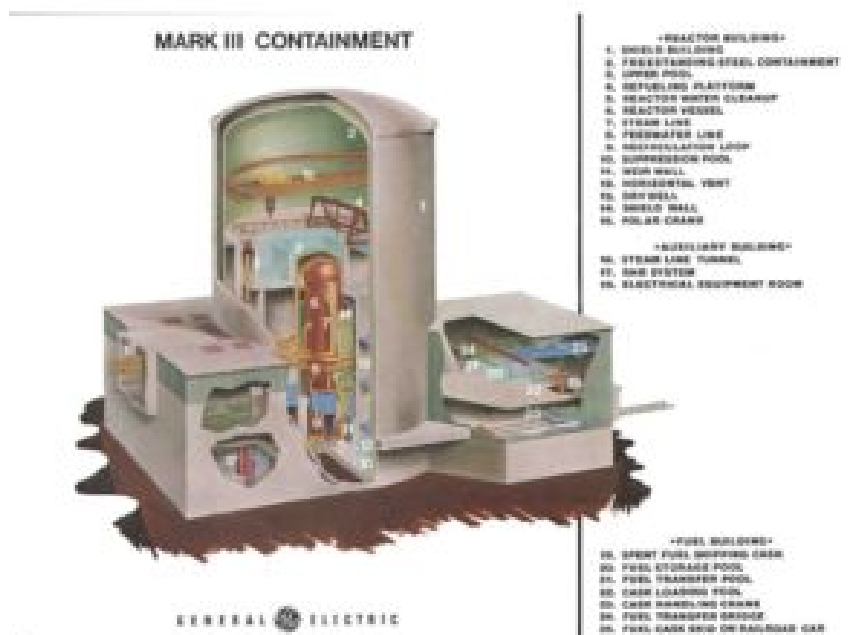
Figure 3: GE Boiling water reactor, Mark III design. Spent fuel pool is to the right of the reactor, number 20, outside the main containment. From NRC, undated.
