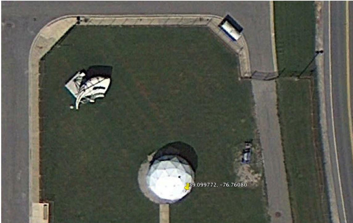
ATCi Model Simulsat 5 C/Ku, precision series multibeam antenna with 70-degree arc, capable of receiving satellite transmissions from 35 or more satellites simultaneously without adjustment or degradation in performance from one satellite to the next, no less than 2-degree compliant with the ability to capture signals from all C and Ku Band satellites within a 70-degree view arc. Frequency: C Band 3.4-4.2 GHz and Ku Band 10.7-12.75 GHz.<sup>60</sup>
