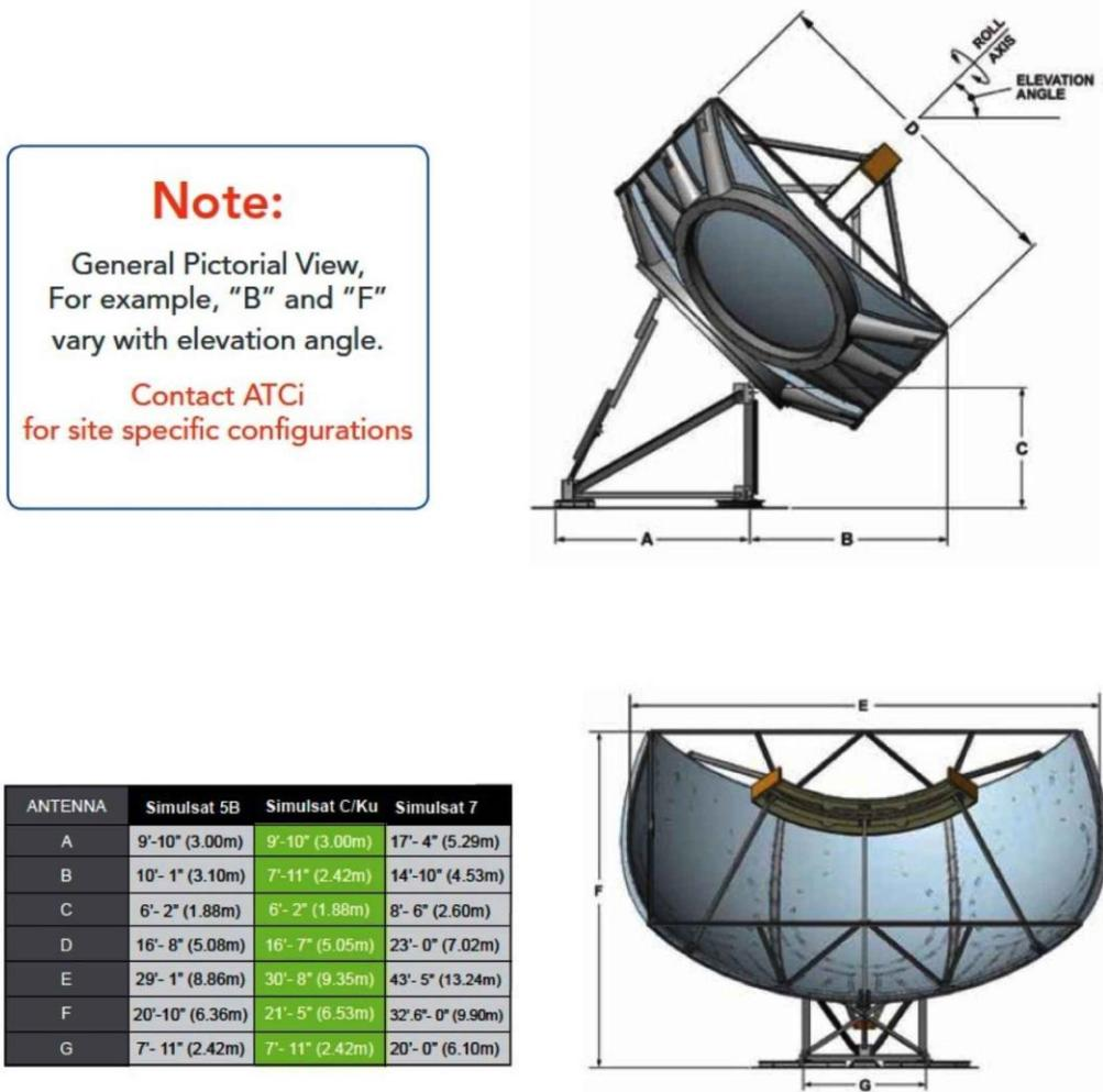
Source: Simulsat Multibeam Earth Station Product Family, (ATCi, 2012), at [http://www.atci.com/assets/simulsat\\_brochure2012.pdf](http://www.atci.com/assets/simulsat_brochure2012.pdf).
